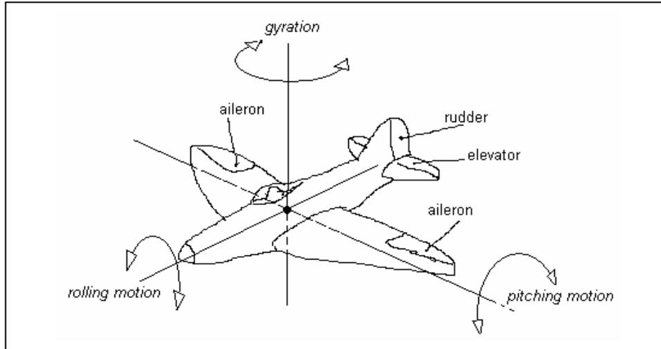
**Fig. 5.2.2** The airplane and basic controlled movements
