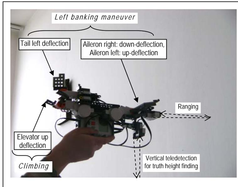
**Fig. 5.2.7** An instance of demonstration with annotated effects
