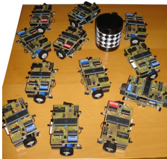
Fig. 1. A swarm of prototype HERD robots is shown. Each robot has a size of 8x12x5 cm. All robots within direct line of sight are able to communicate by infrared senders and receivers.
