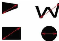
Fig. 2. How to measure robot foot dimensions
