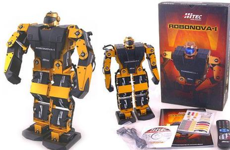
Fig. 3. The ROBONOVA-I platform
