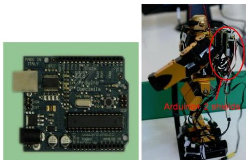
Fig. 4: The Arduino board (left) and the board with two 'shield boards' integrated in a ROBONOVA robot (right)
