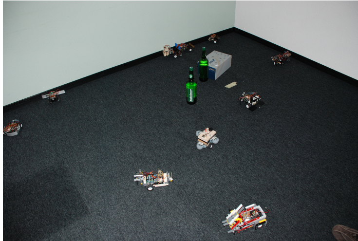
Fig. 4. The environment with all the predator and prey robots together. The green bottles and the card box are the obstacles. The ground had dark color and the hideout was a white paper (not seen in this picture).
